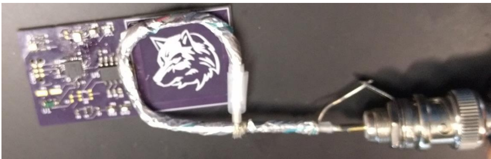
Figure 4.8: Loop Probe for Antenna Tuning
