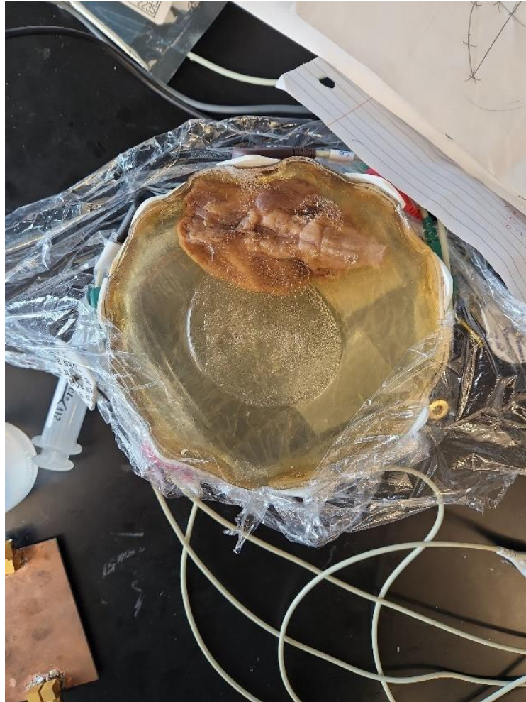
Figure 8.4. Lamb brain tissue embedded in a tissue phantom
