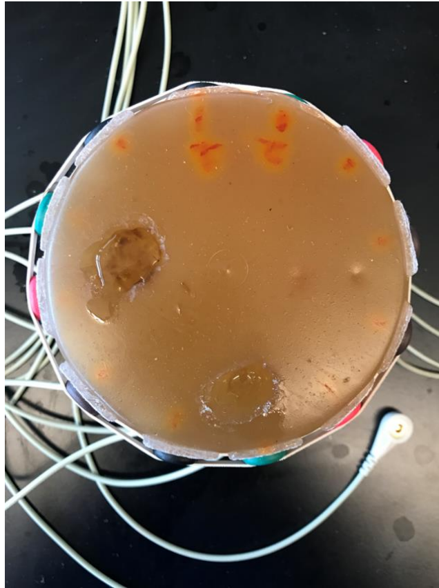
Figure 4.15. Phantom image, homogenous data. For inhomogenous data, the left hole was filled and the bottom one was emptied.
