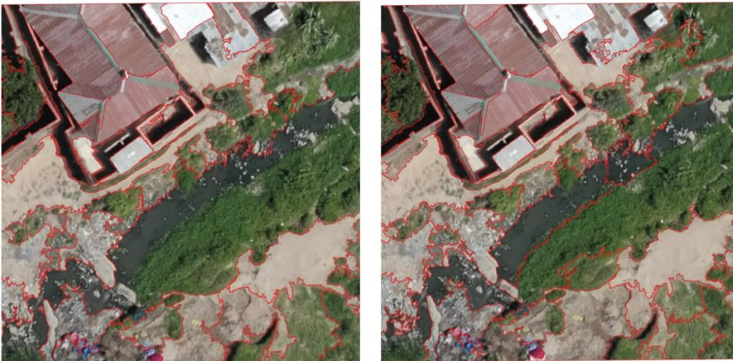
Figure 7. Comparison of segments with spectral radius of 50 radiometry units, the image to the left was developed using a range radius of 30 radiometry units while the image on the right was created using range radius of 25 radiometry units.
