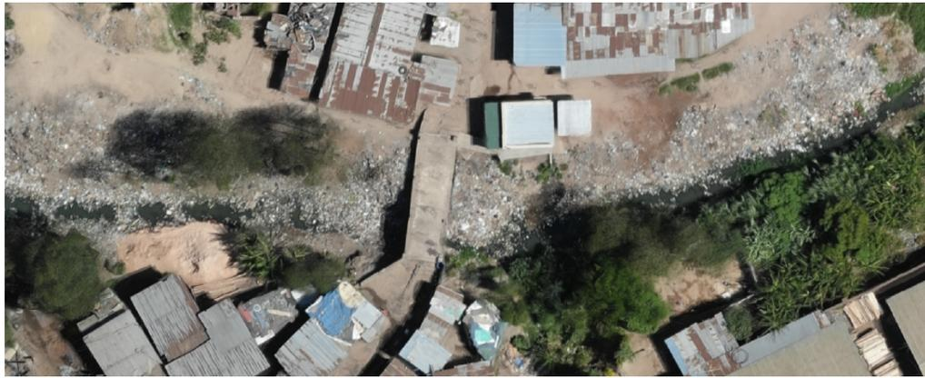
Figure 6. Waste pile seen in the Clipped UAV imagery captured with a GSD of 3.79 cm.
