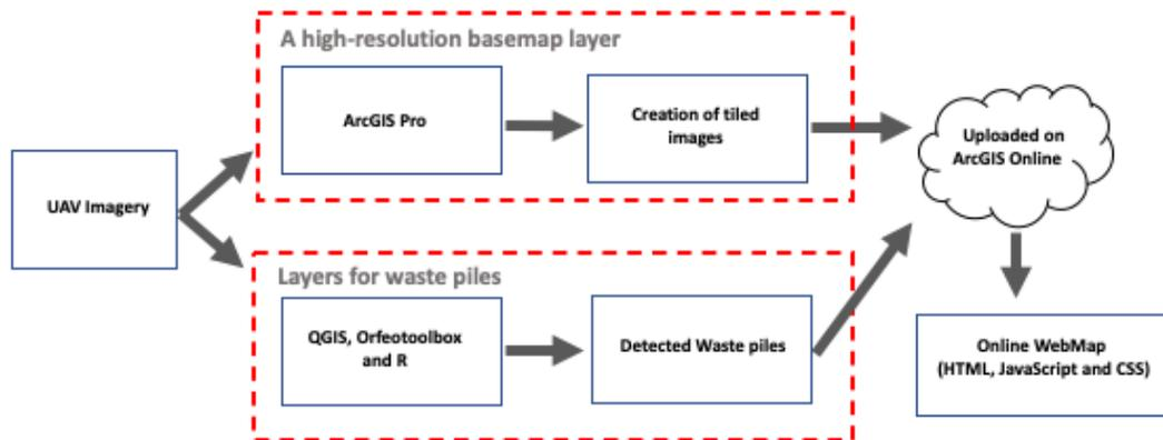
Figure 8. The workflow for development of the web application for waste pile locations.
