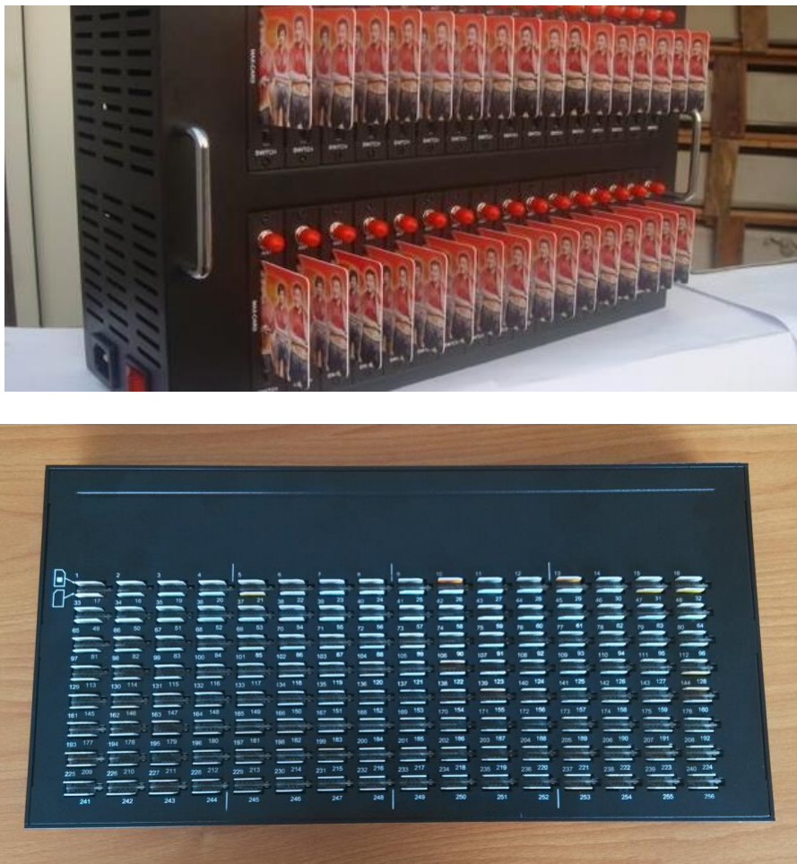
Figure 6: Two models of actual Simbox devices (Weddi, 2015; Angela Wu Huizhou Yuexun Network Technology Co., Ltd, 2016)
