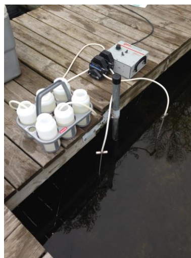
Figure 2.3. Water sampling methods of groundwater at each lake site. A piezometer was pushed through the sediment until the aquifer was detected. The piezometer was then attached to a peristaltic pump to draw groundwater to the surface and into sample bottles.
