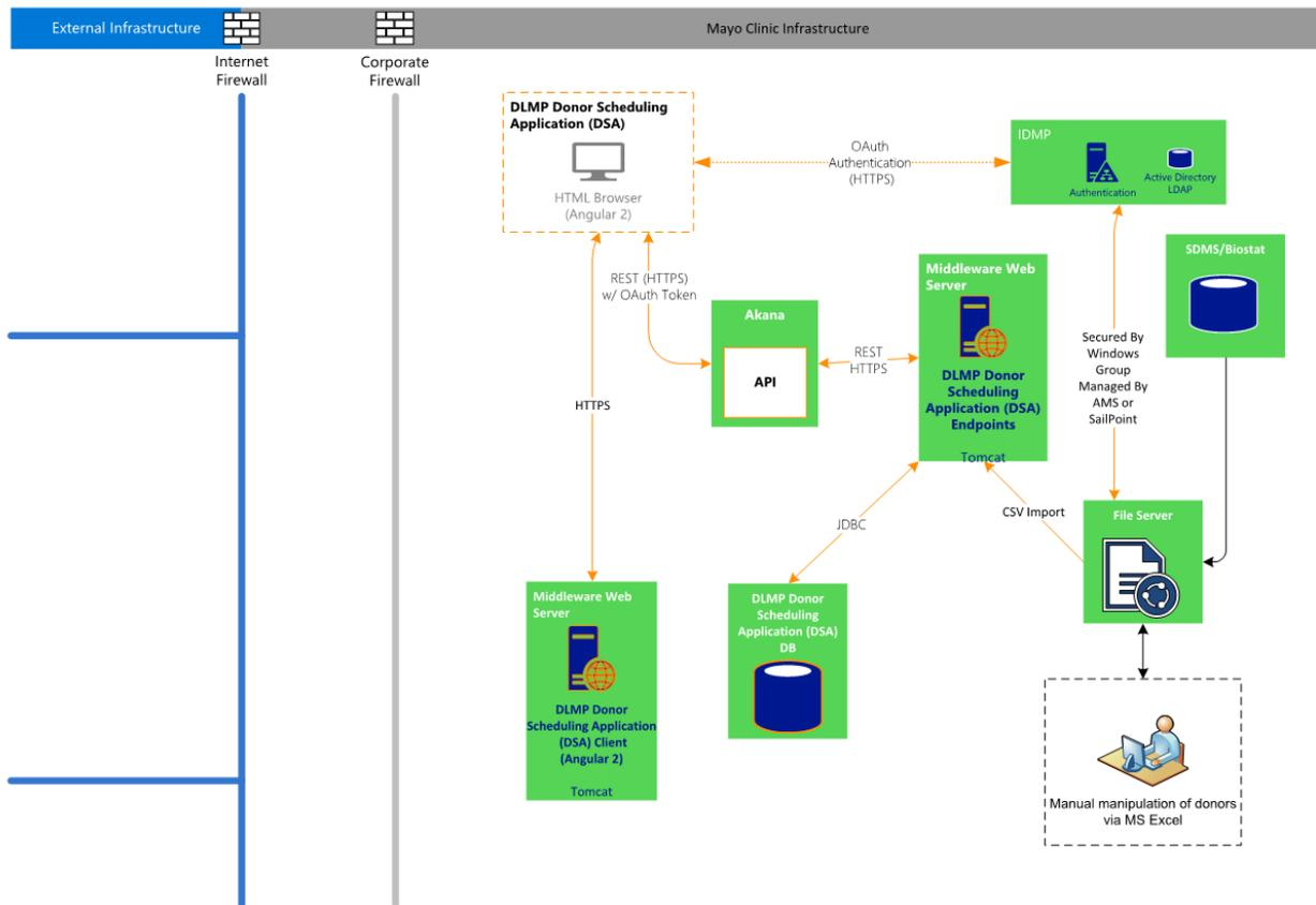
Figure 7: DLMP – DSA – System Architecture
