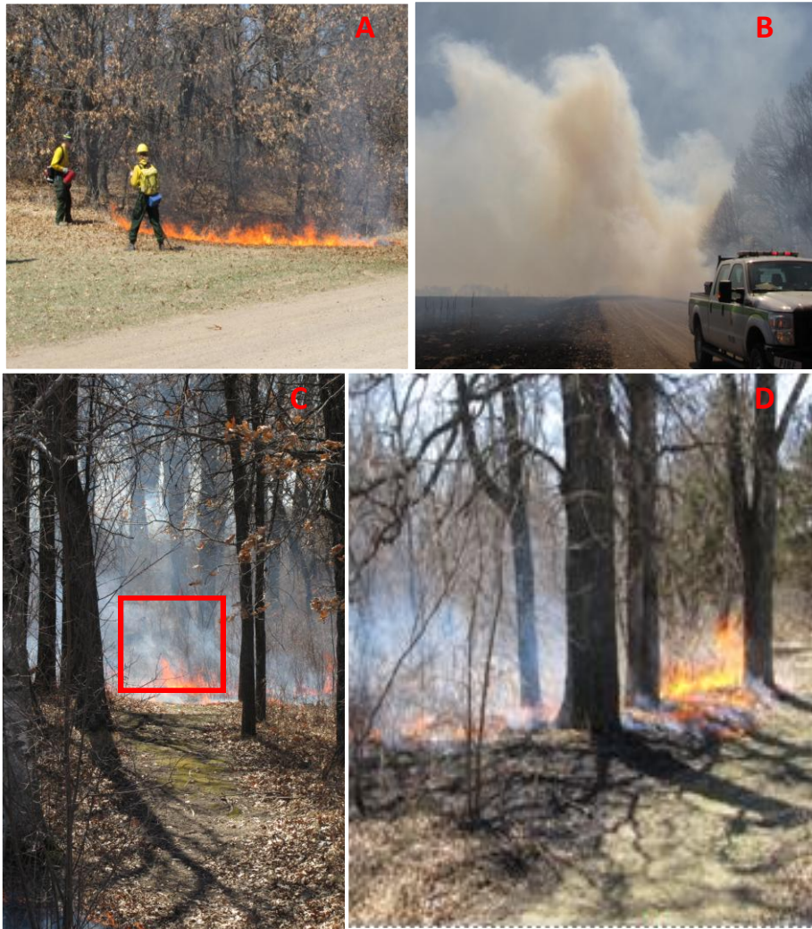
Figure 4. A, Photograph of initial ignition. B, Photograph of smoke column generated by burn approximately 10 minutes after ignition. C, Photograph of fire beginning to encroach on test plot area. D, Photograph of fire in area near test plot. Note fire is mostly creeping through the oak litter with limited flame height.
