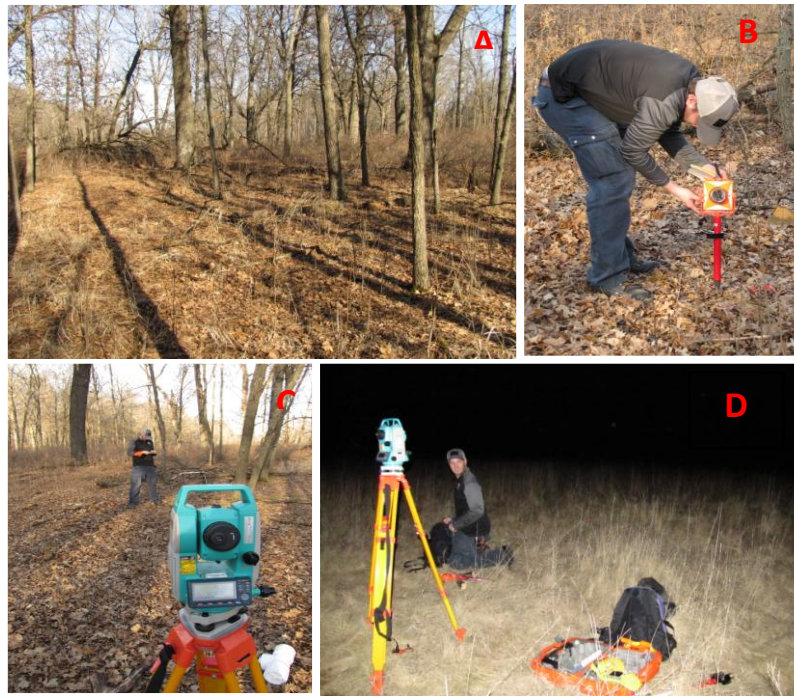
Figure 2. A, Overview of first attempt in woodland habitat. B, Ian Hanson holding Stadia Rod on top of artifact to be mapped. C, Ian Hanson and Total station used for mapping. D, Ian Hanson and equipment after mapping first attempted grassland plot.
