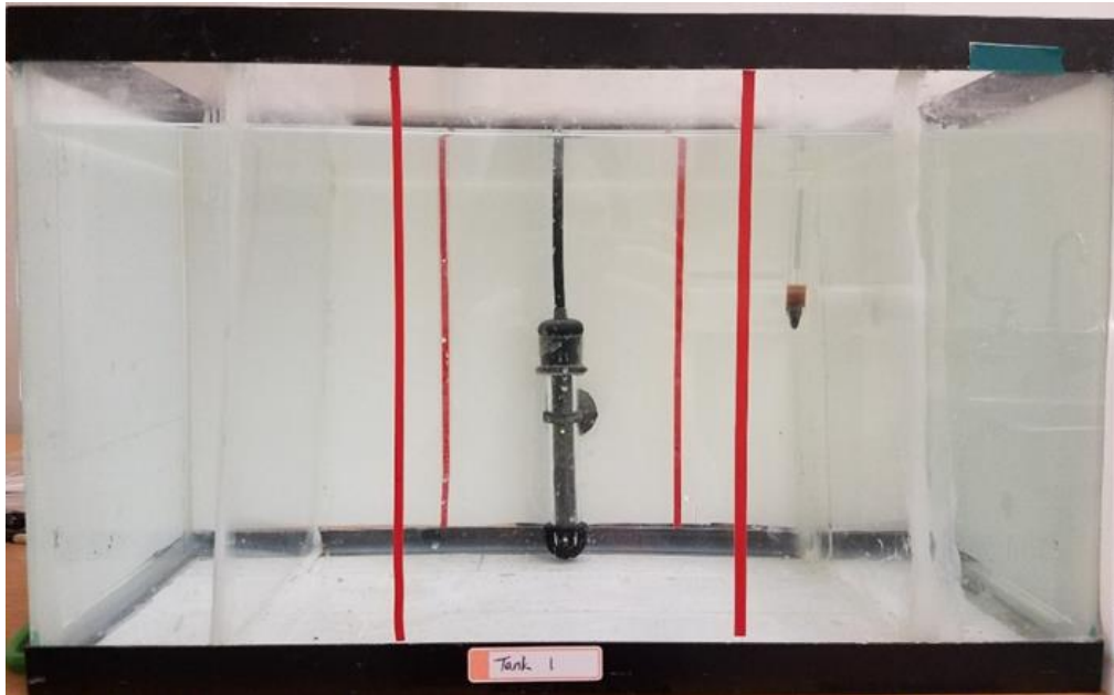
Figure 2.3. Test Apparatus Front View. The red lines indicate the edge of preference zones with the center of the tank reserved as the indifference or neutral zone. The males are contained by clear plexiglass dividers on opposite ends of the tank.
