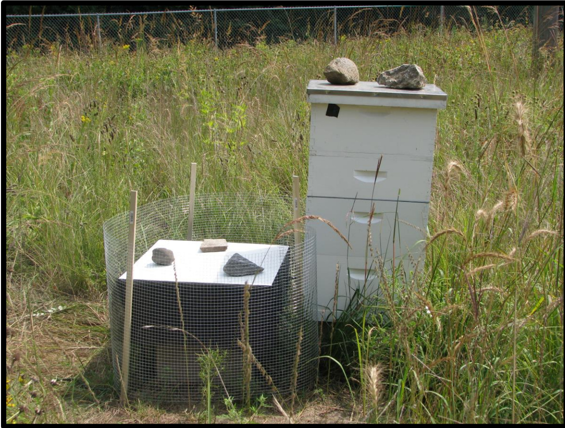
Figure 6.3. Experimental hive surrounded by (1.5 cm diameter openings) a chicken wire fence to act as a Faraday cage to mitigate any harmful unwanted exposure to high frequency waves.
