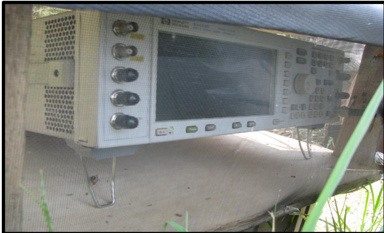
Figure 5.3. Hewlett Packard E4433B digital RF Signal Generator (250 kHz- 4 GHz) with 2.4 GHz rubber ducky antenna attached. Unit is housed within a pine box for weather protection during 30 day continuous exposure.
