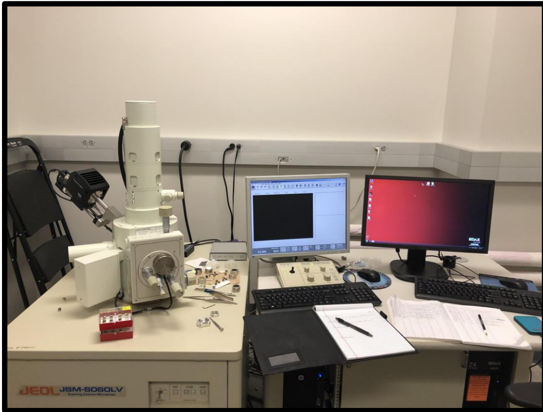
Figure 10.3. Scanning electron microscope and energy dispersive X-ray spectrometer work station for particle abundance analysis.
