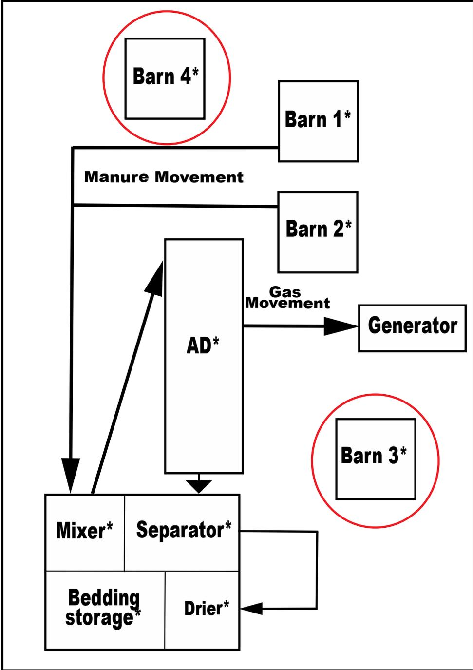
Figure 2.1. Haubenschild farm schematic, anaerobic digester (AD) set-up, and main sampling points (\*). Arrows indicate manure movement from barns to the digester through the mixer and the return of the digester through the separator, drier and ending up at the bedding storage section. Barns 3 and 4 (circled) are isolated and don't contribute to the anaerobic digester
