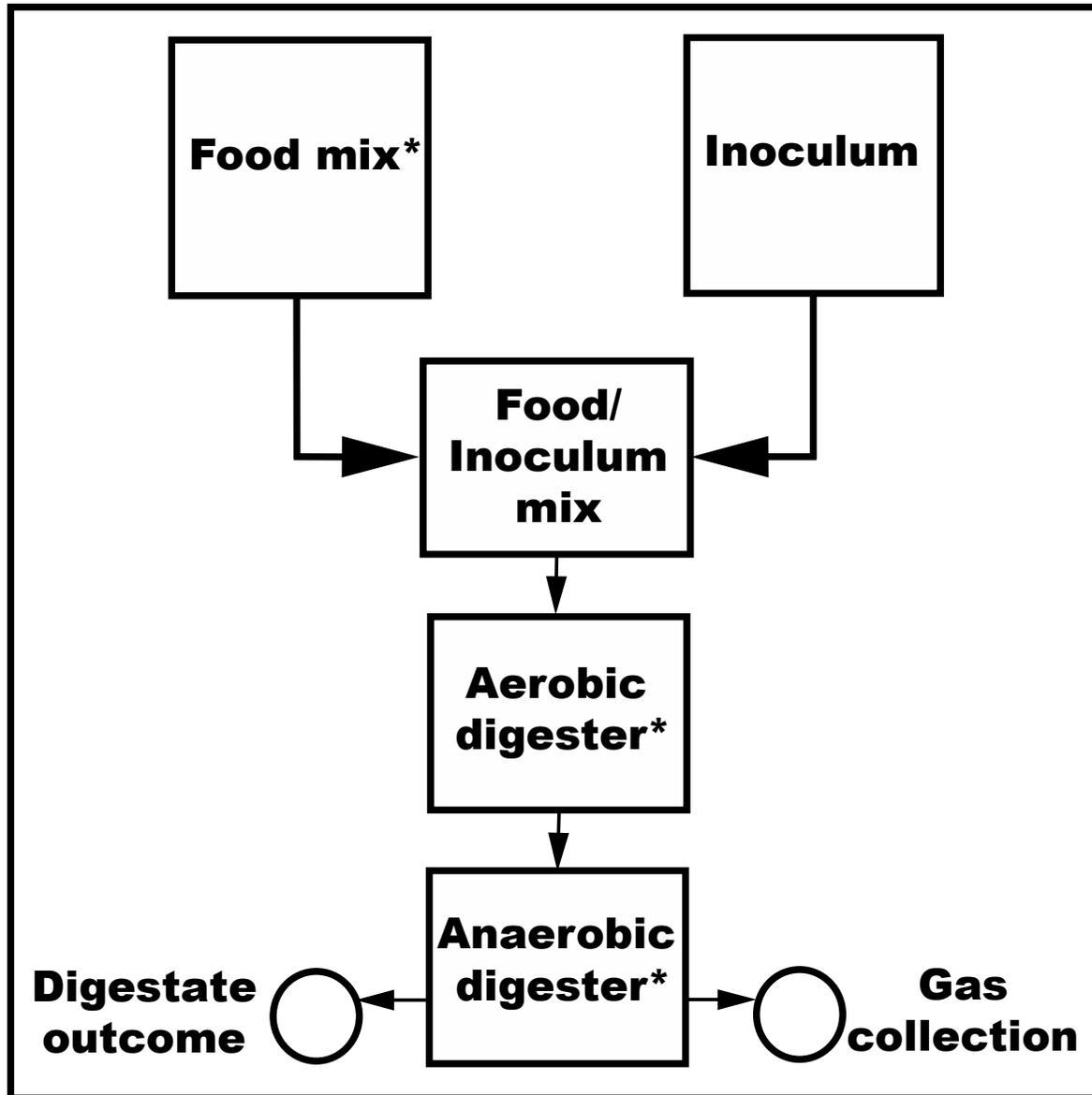
Figure 2.12. University of Minnesota, experimental benchtop AD set up; main sampling points (indicated by the asterisks \*).
