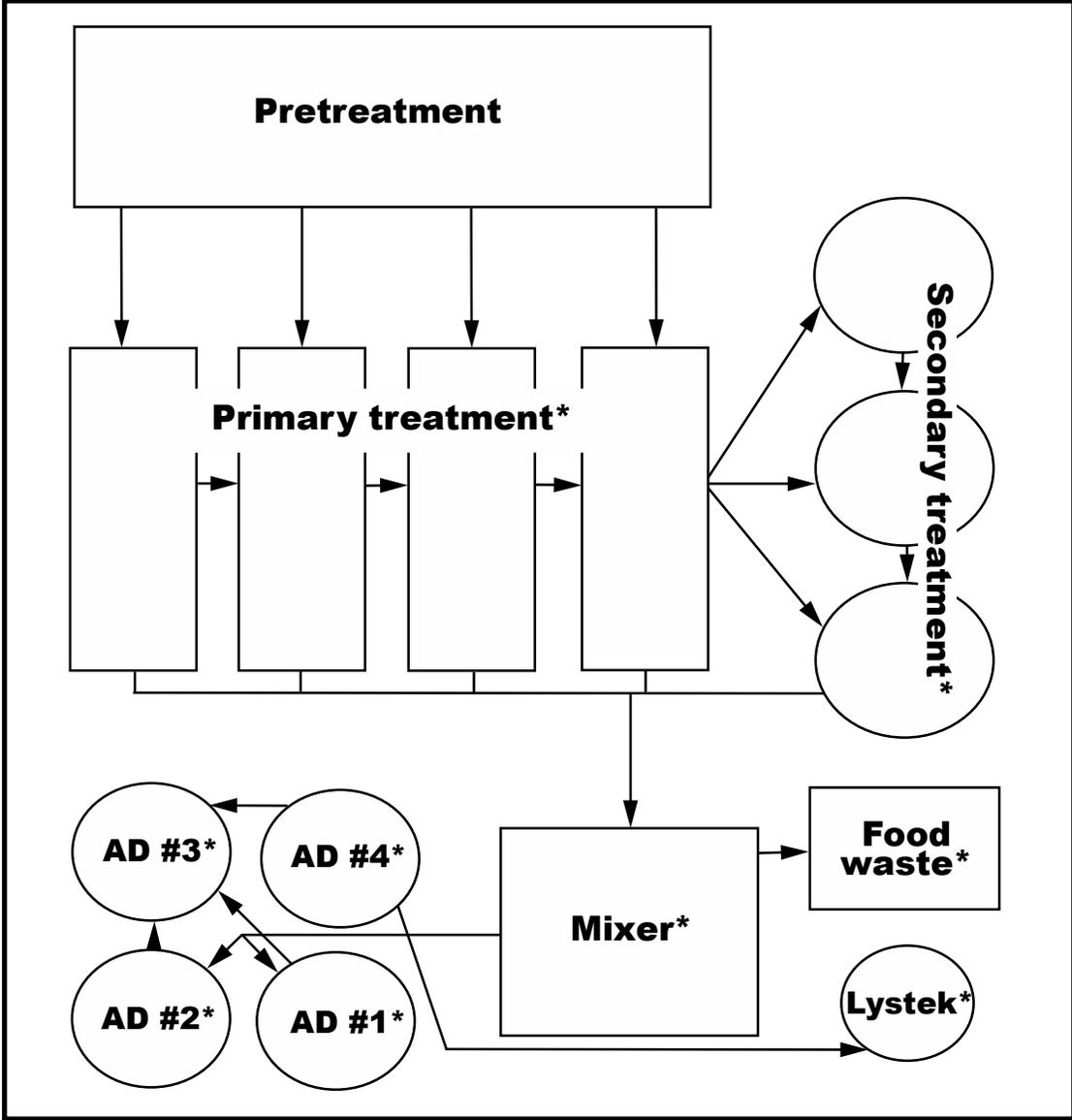
Figure 2.7. ST Cloud WWTF schematic, including AD set-up and main sampling points (indicated by the asterisks \*).
