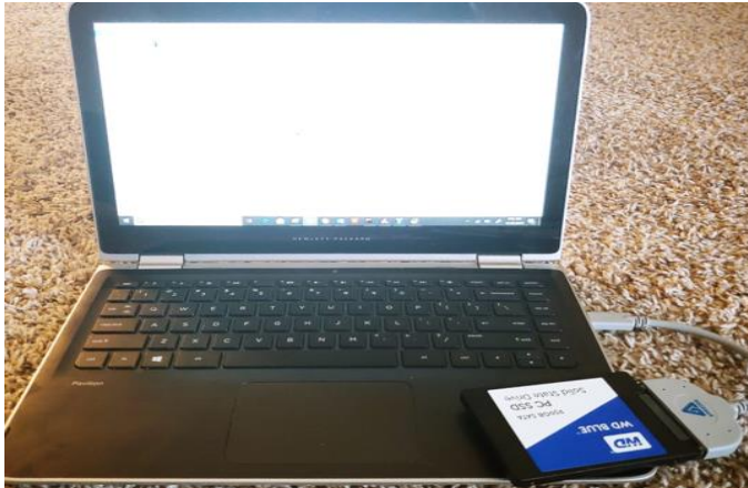
Figure 31. Internal SSD Connected Externally to a System Using ESATA Port
