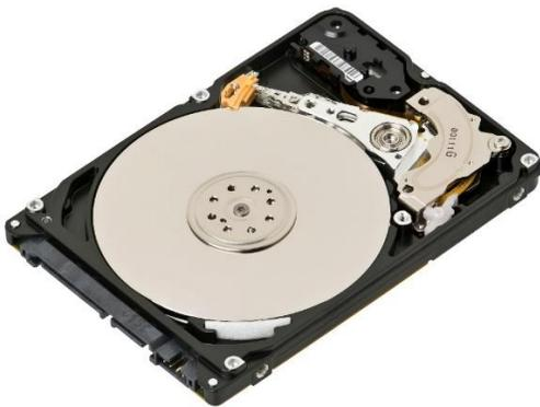
*Figure 2.* Hard Drive (Phelps, 2012)
