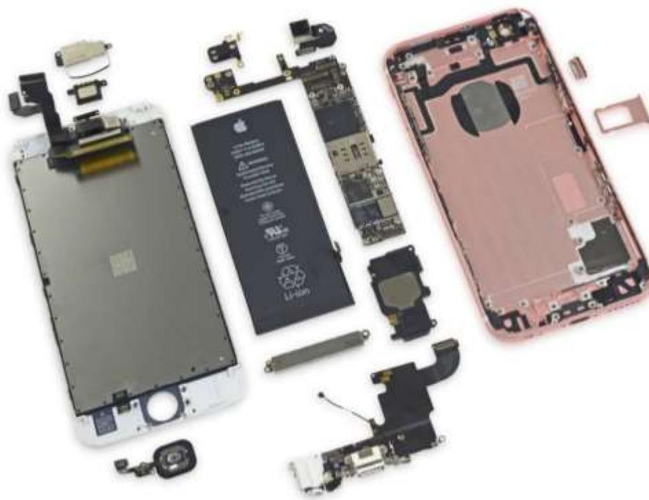
Figure 4: Dismantled components of an iPhone 6s (ifixit, 2015)
