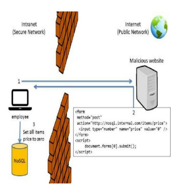
Note. A depiction of how CSRF can be performed via NoSQL REST API (Aviv et al., 2015)
