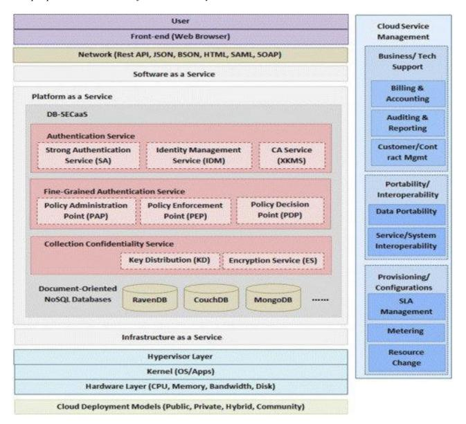
Note. The proposed architecture of DB-SECaaS system over a document-oriented database hosted in the cloud (Ghazi et al., 2016)
