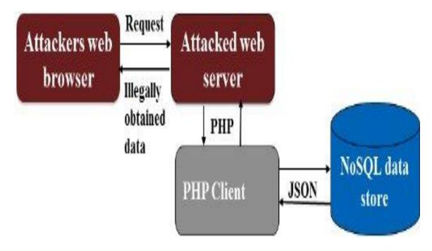
*Note*: A representation of the architecture of a PHP web application (Aviv et al., 2015)
